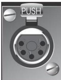
This is a 5-Pin female XLR connector used to connect a microphone and push-to-talk(PTT) switch. The ProTraXX can route the microphone input to any channels or group of channels. See the section on “*Microphone Paging*” for additional details.
