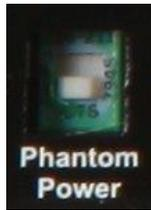
Setting this DIP switch to the ON position enables phantom power (48V) on the microphone input.
