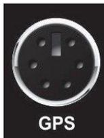
The 6-pin mini-DIN connector is used for GPS connection. When a valid GPS source is connected and satellite lock is achieved, ProTraXX will use the GPS time to set the system clock once an hour. While using GPS to sync the system clock, make sure the time zone and daylight savings time mode is properly set on the unit. The ProTraXX accepts a standard NMEA-0183 data stream at 4800 baud.
